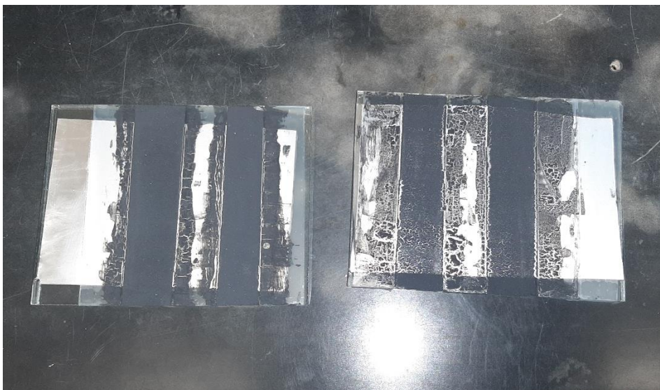
Figure 37: a smooth and thick active layer coat on foil paper (left) vs uneven and cracked active layer coat on foil paper (right)
