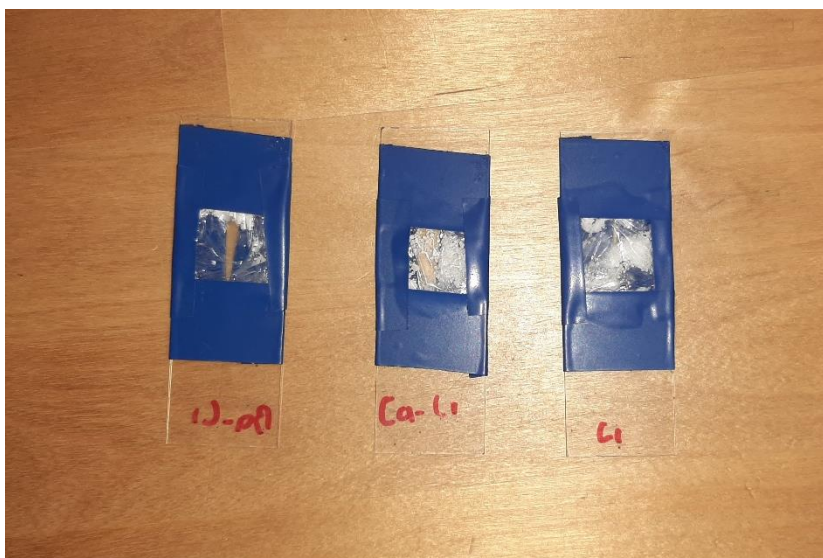
Figure 11: Samples covered with plastic foil for X-ray diffraction
