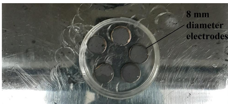
Figure 38: 8mm diameter punched electrodes with active layer coat
