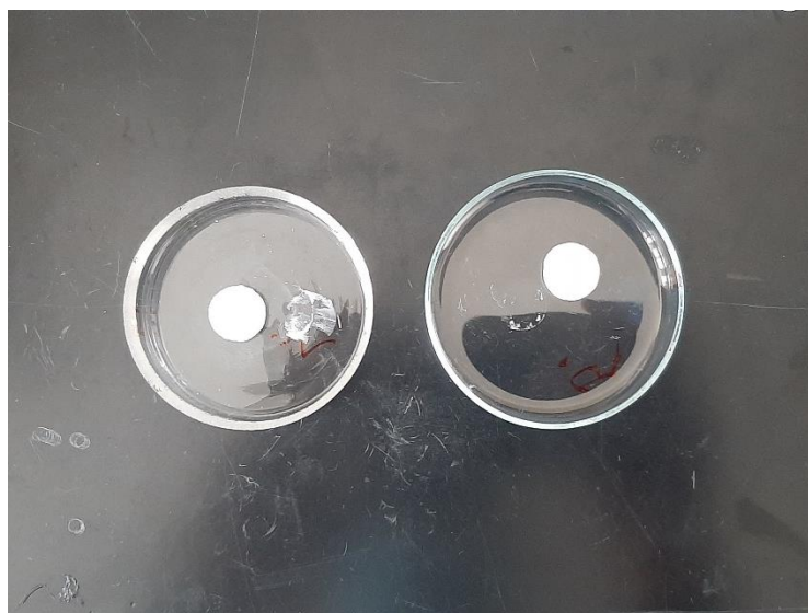
Figure 39: electrolytes compressed into pellets for coin cell assembly
